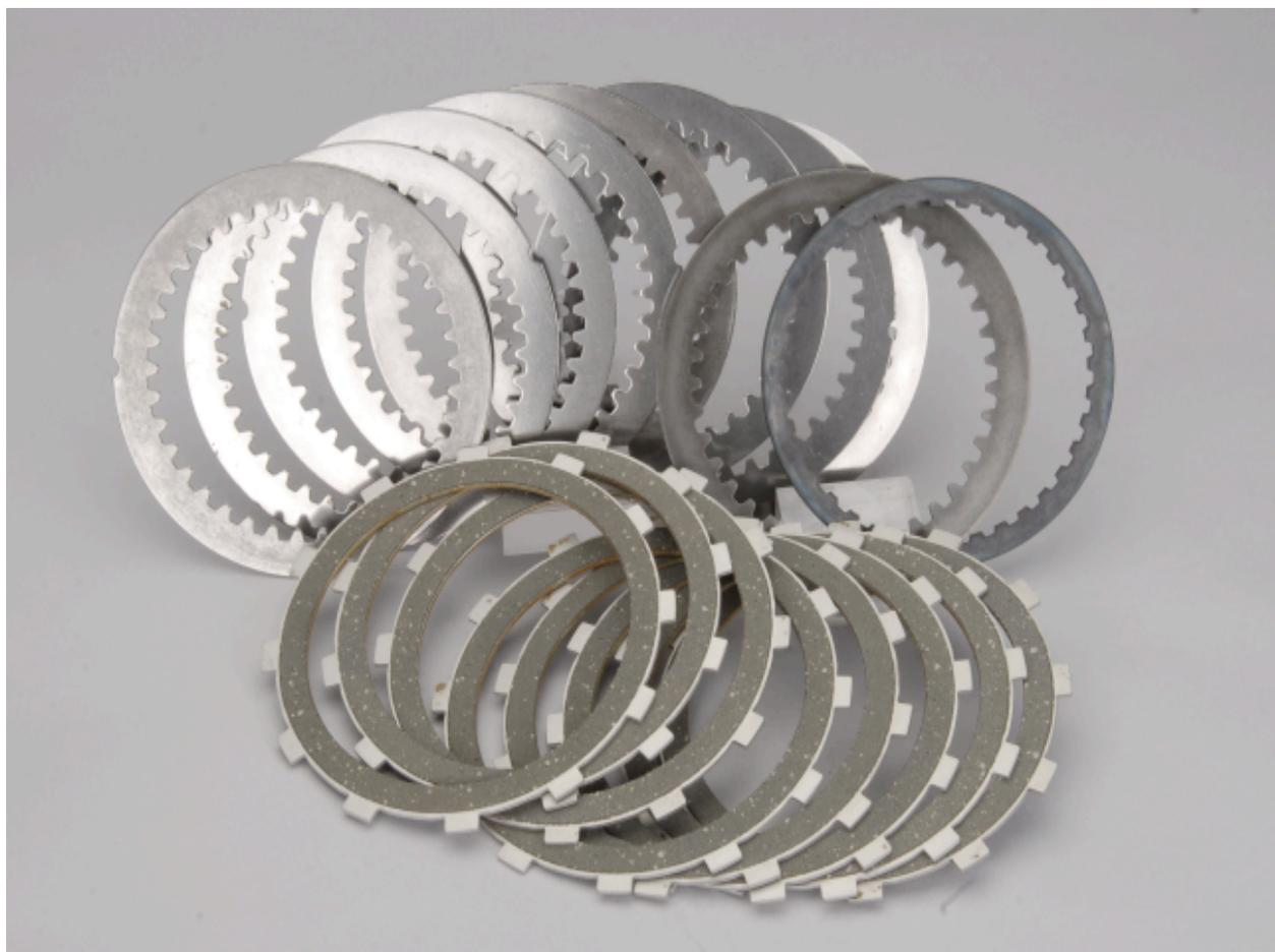
Our clutch kits have been designed to improve the feel and durability of the clutch. These kits usually have two more plates than the oe clutch. In this way, the friction surface is correspondingly increased, and the torque load on each plate reduced.
